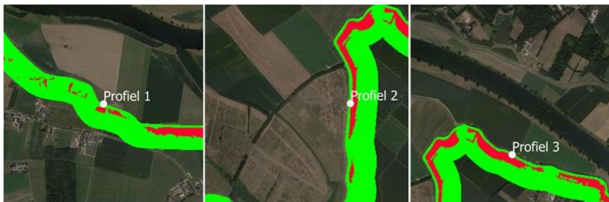
Figure 10: Piping ter plekke van 3 doorsnedes
